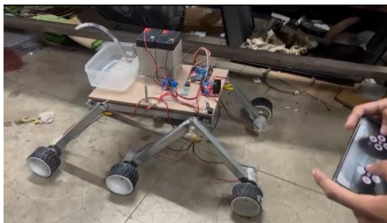
Fig. 2 ROCKER BOGIE FIRE RESCUER DEVELOPED MODEL
