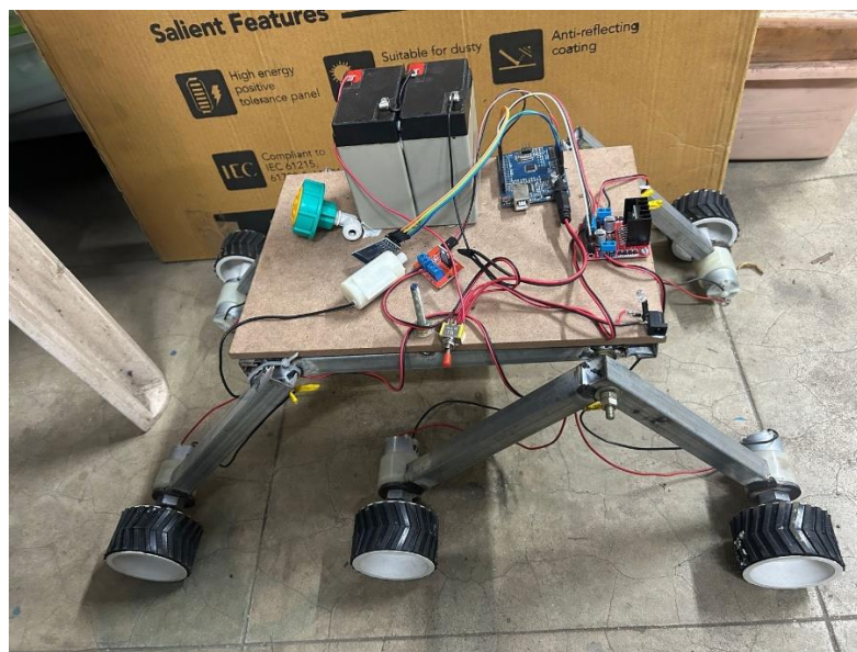
Fig. 1 ASSEMBLY VIEW OF ROCKER BOGGIE FIRE RESCUE
